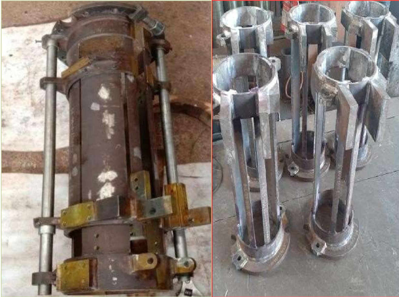
Mobile & Immobile Tube Structure- Material-IS 2062 E250
