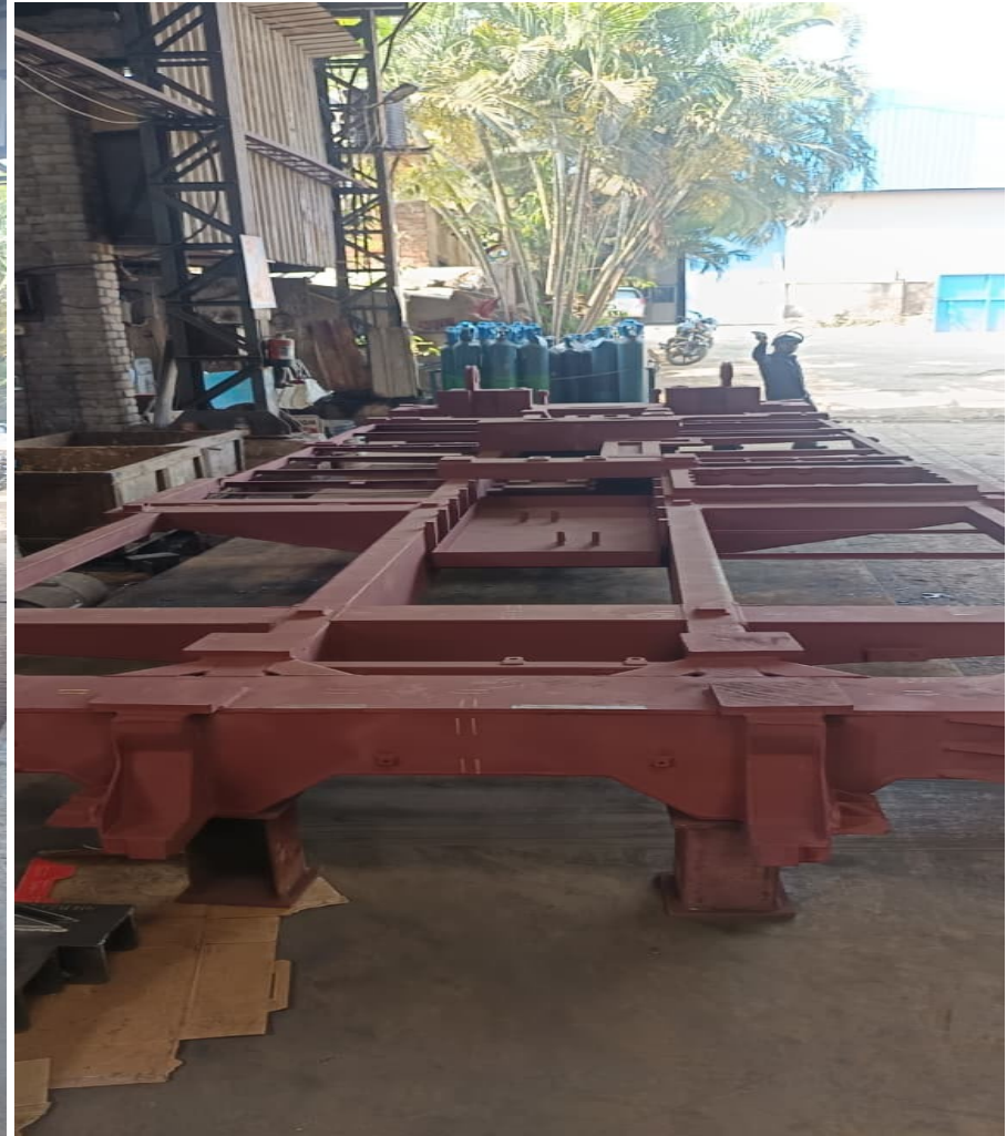
MRSAM & ASAM – UNDERFRAME STRUCTURE WELDED MATERIAL:- EN 10025-6-S690QL SIZE:- 8000 X 2286 X 1000
