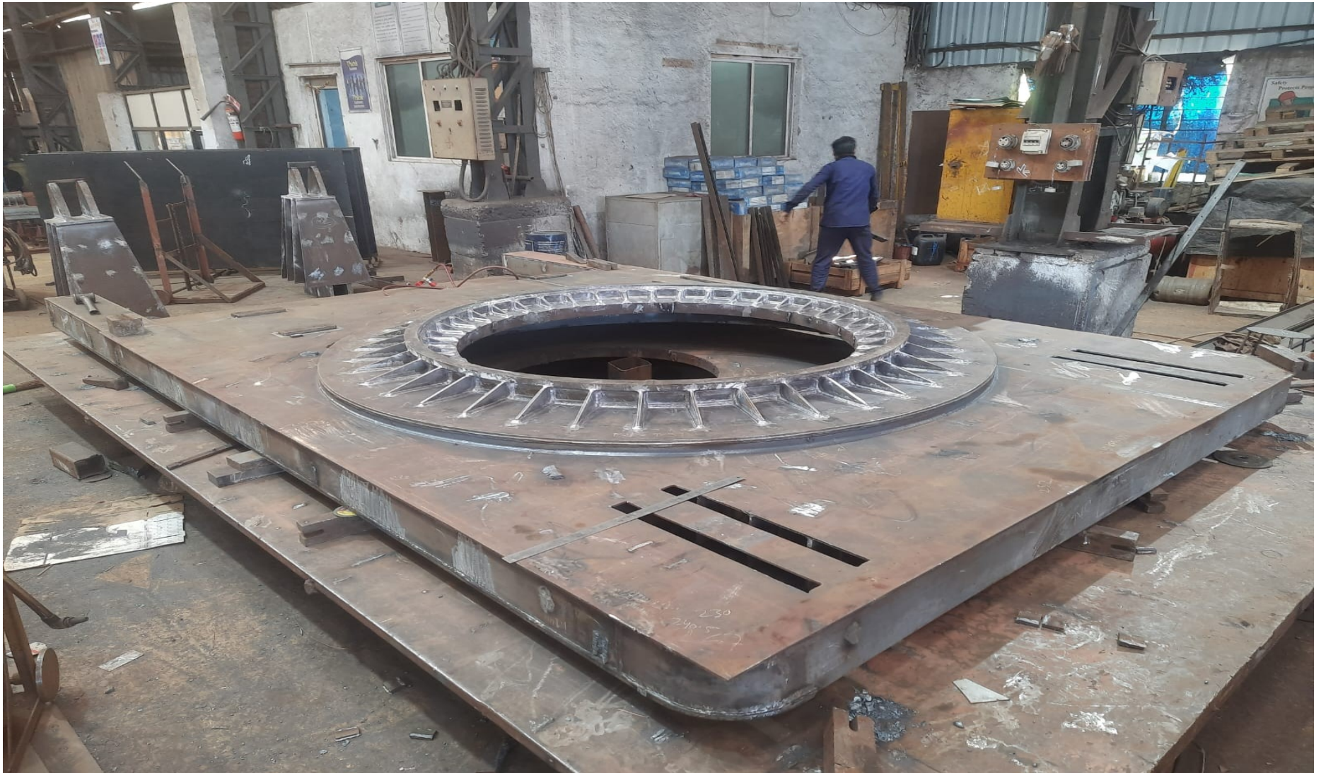
FCR : ROTARY PLATFORM STRUCTURE MATERIAL:- S690QL / SIZE:- 5000 X 2660 X 500
