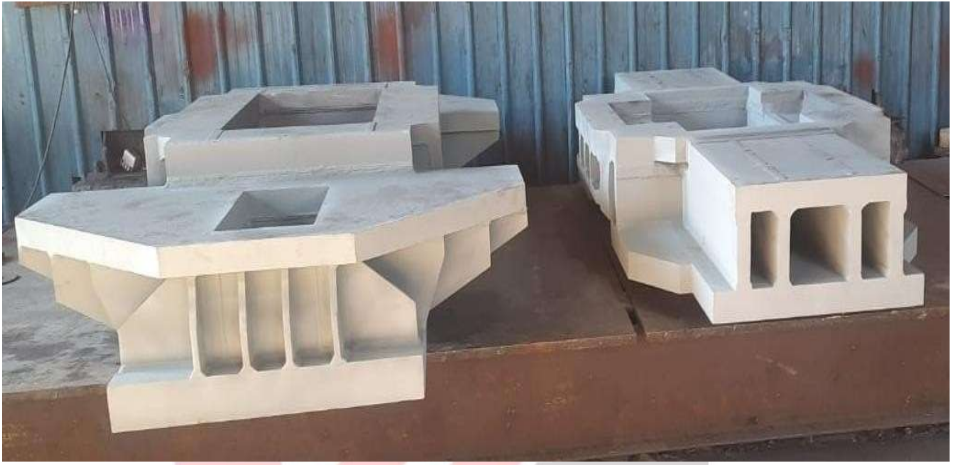
Upstream Structure & Downstream Structure- 5000 X 2000 x 350-Material : IS 2062 E350C
