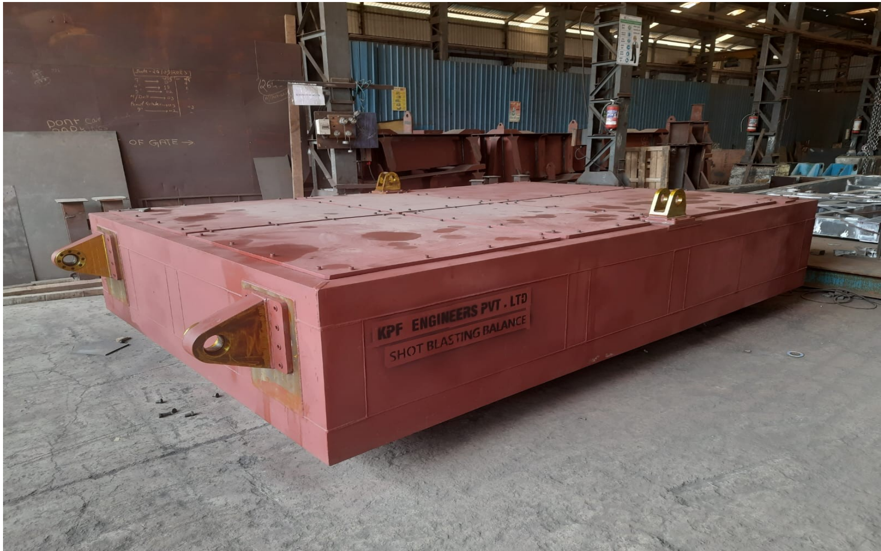
FCR : DUMMY ANTENA MATERIAL:- S690QL / SIZE:- 4500 X 2500 X 450
