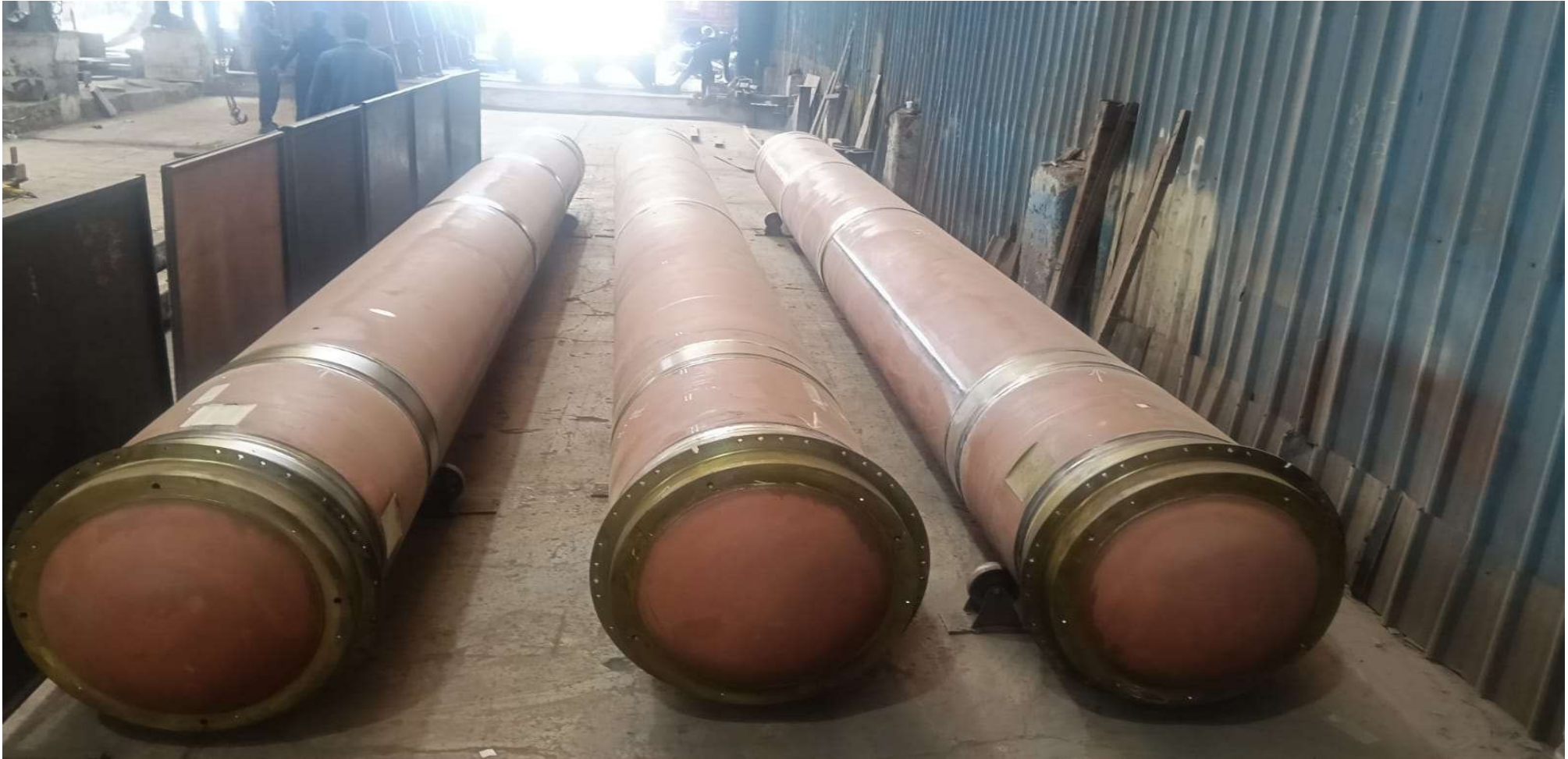
TCIL - DUMMY CANISTER ASSY MATERIAL- IS 2062 = 9000mm X 2000mm DIA
