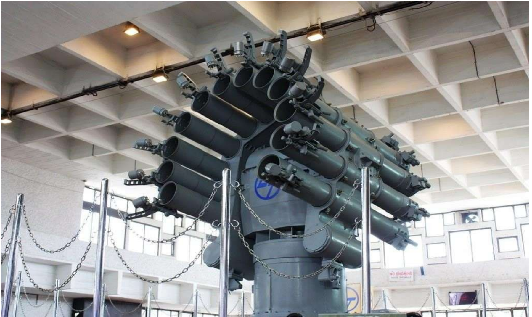
Indigenous rocket launcher-Material DMR 249A, SA 350 LF2 CL2 , CRCA (Refer next 5 pages)
