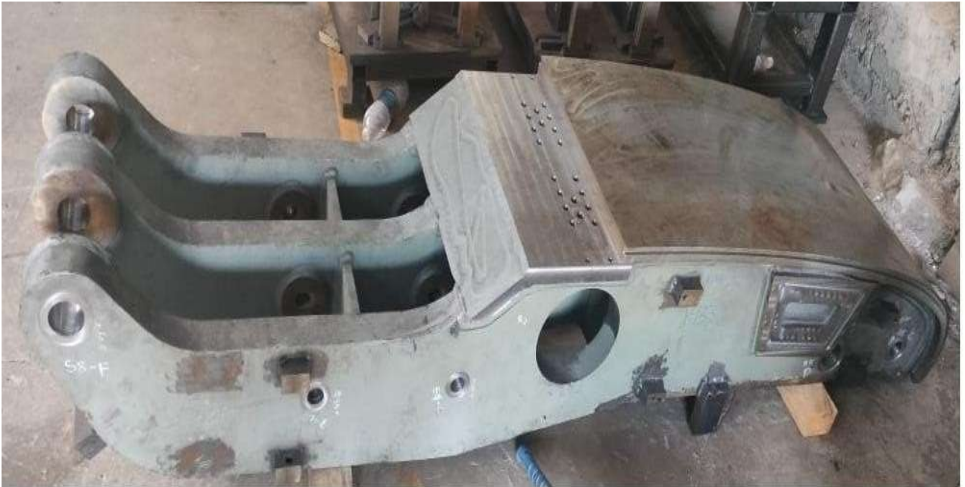
Throat Block- 2500 X 600 X 500 -Material: IS 2062 E350C
