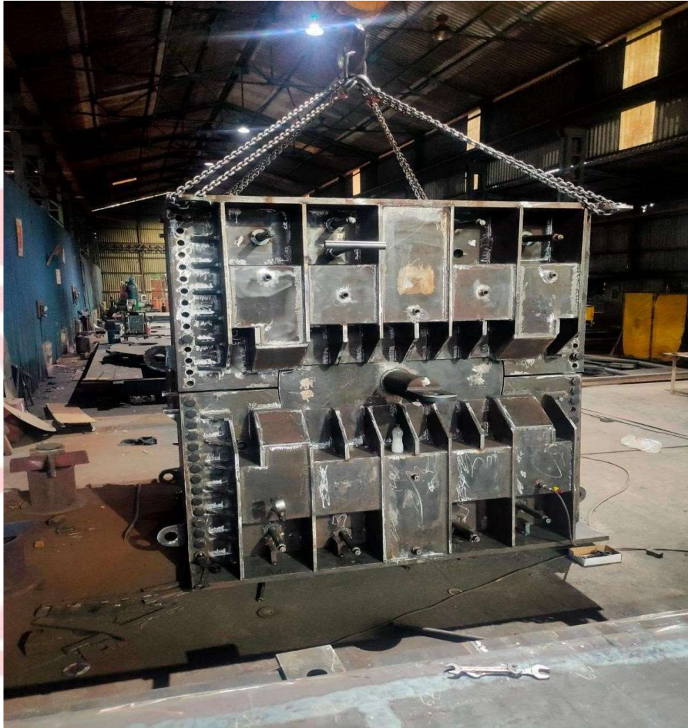
U-mould -3000 mm X 3000 mm X 2500 mm- Material –IS 2062 E250
