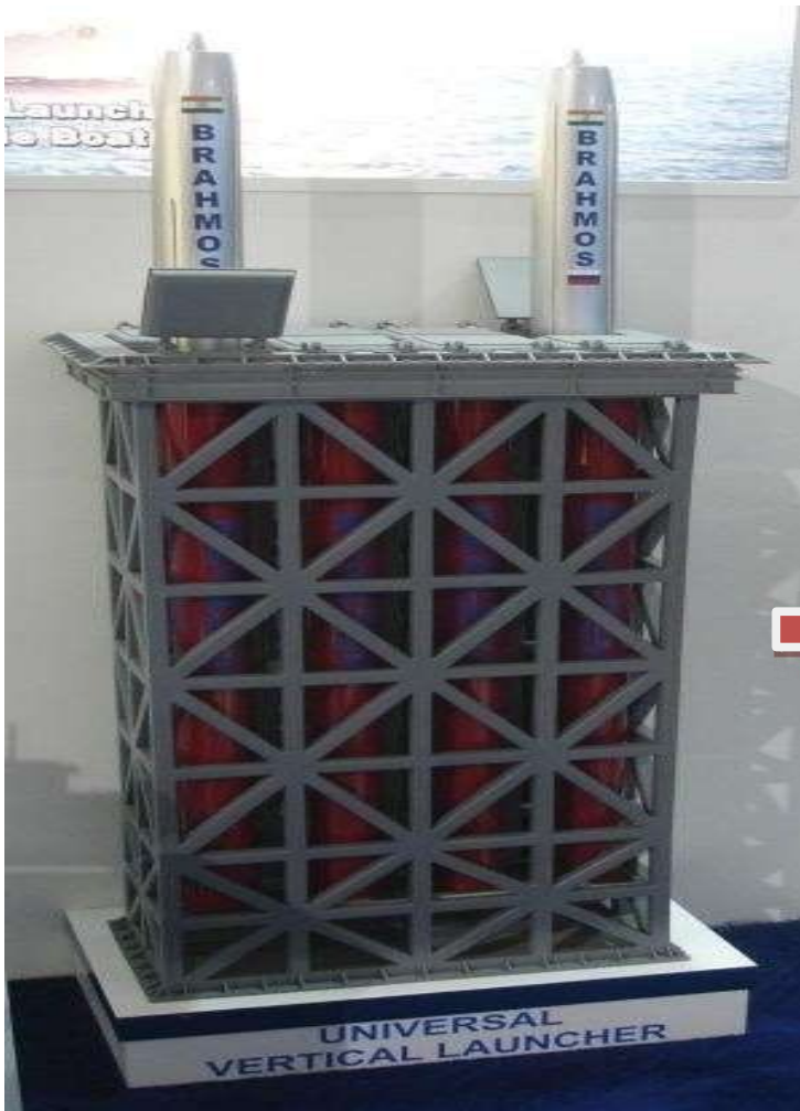
Universal Vertical Launcher Mechanism-Launcher Frame Assembly- 2100 X 4000 X 9000 mm;Material- DMR 249A (Refer next 3 pages)
