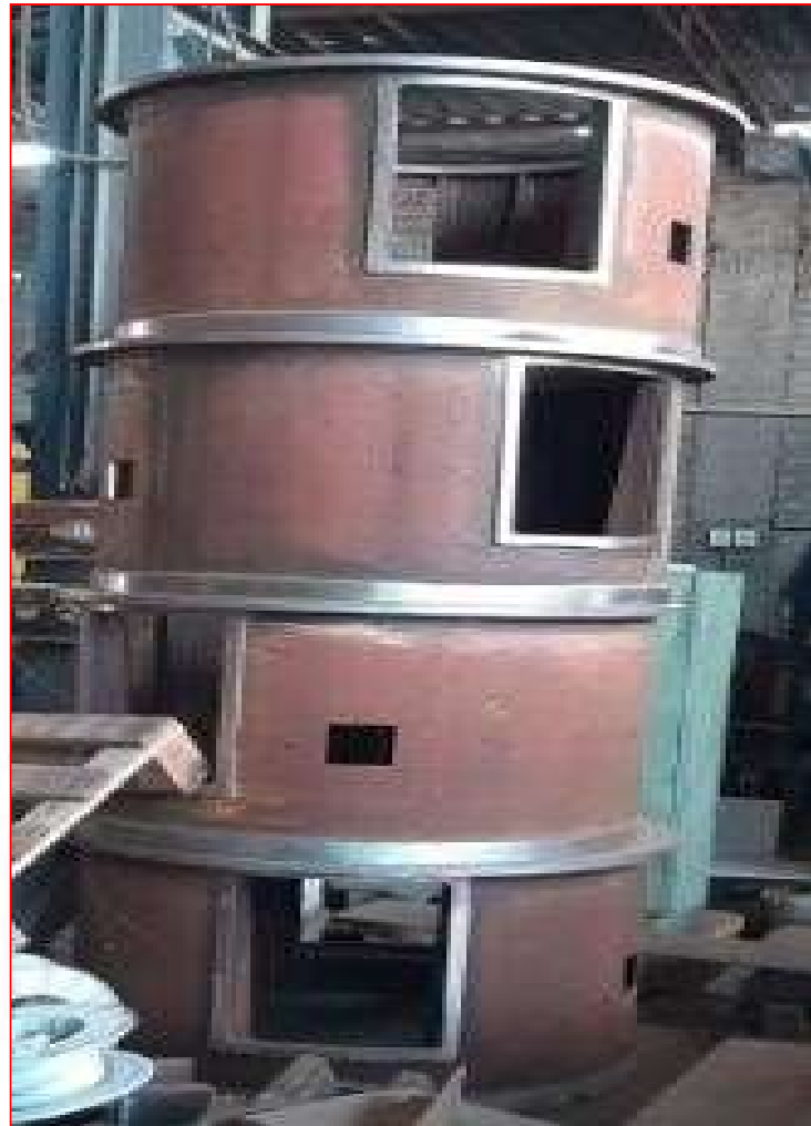
IRL-Stationary Frame- Material-DMR 249A , SA 350 LF 2 CLASS II
