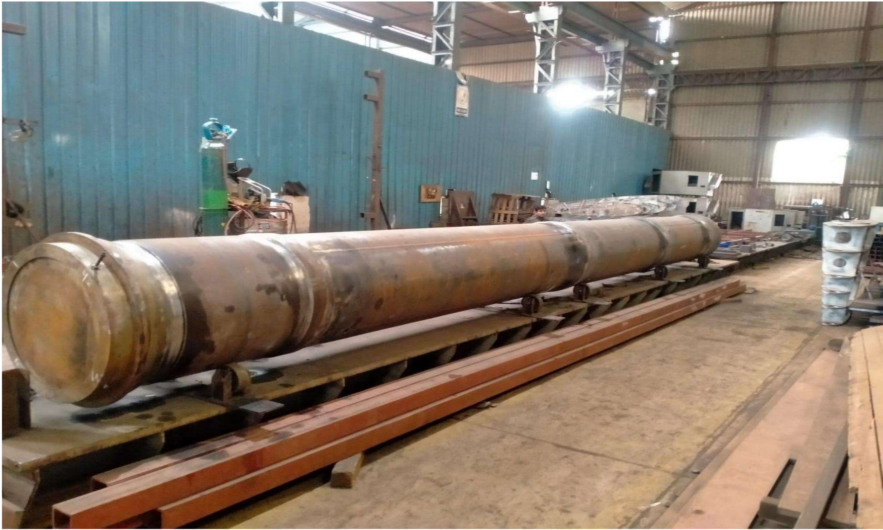
UVLM –Dummy Canister- Material IS 2062 , SA 105 ; Dia. 1000 mm ; 9000 mm Length
