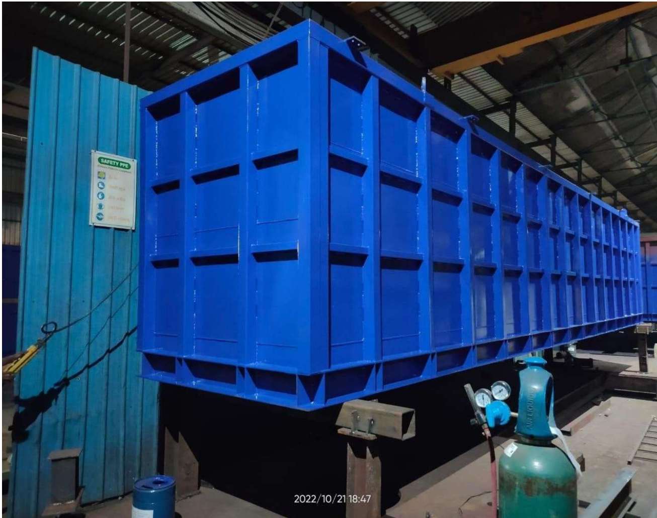
BENTONITE TANK 12000 X 2300 X 2100
