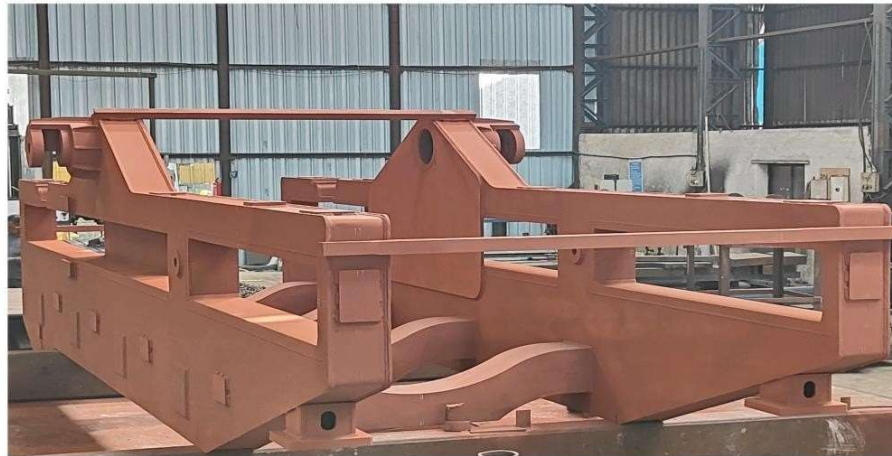
RML TILT BEAM-MATERIAL S690QL- 7000mm x 2500 mm x 3000mm
