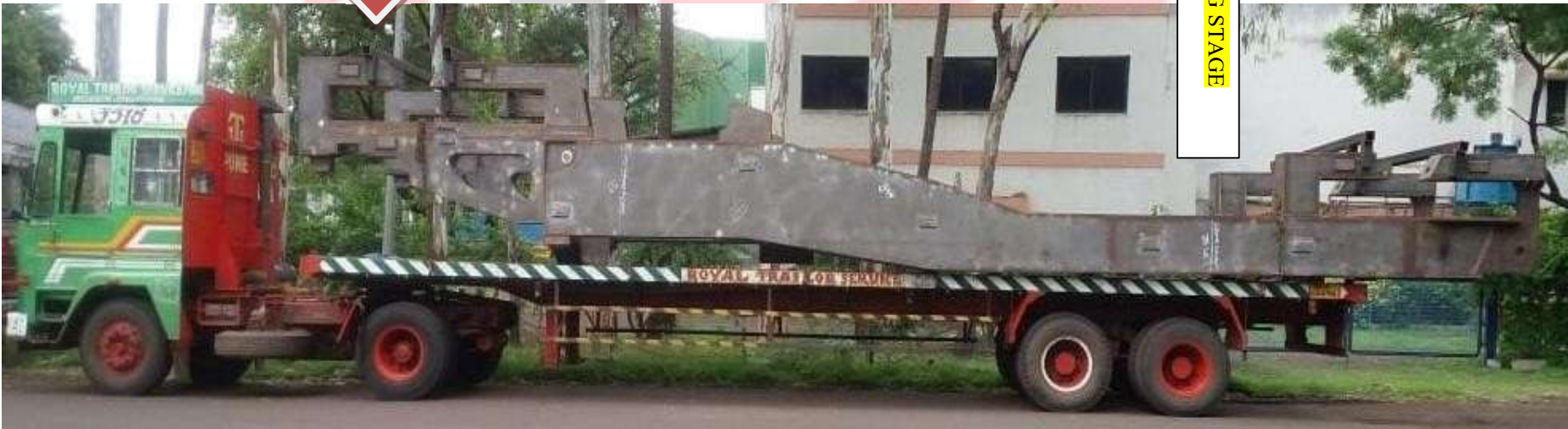
TCT5-Tilt Beam- 3000 x 1300 x 15000 mm Material-IS 2062 E450
