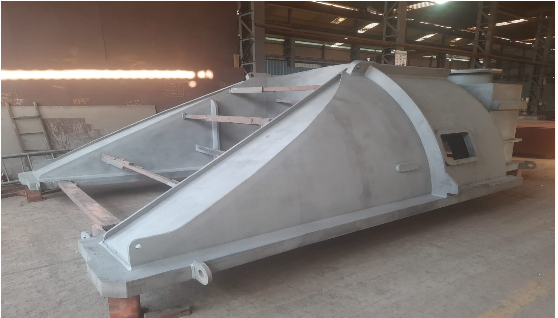
UPPER CASING MATERIAL:- IS 2062 E250 GR BR / SIZE:- 4500 X 2800 X 1500
