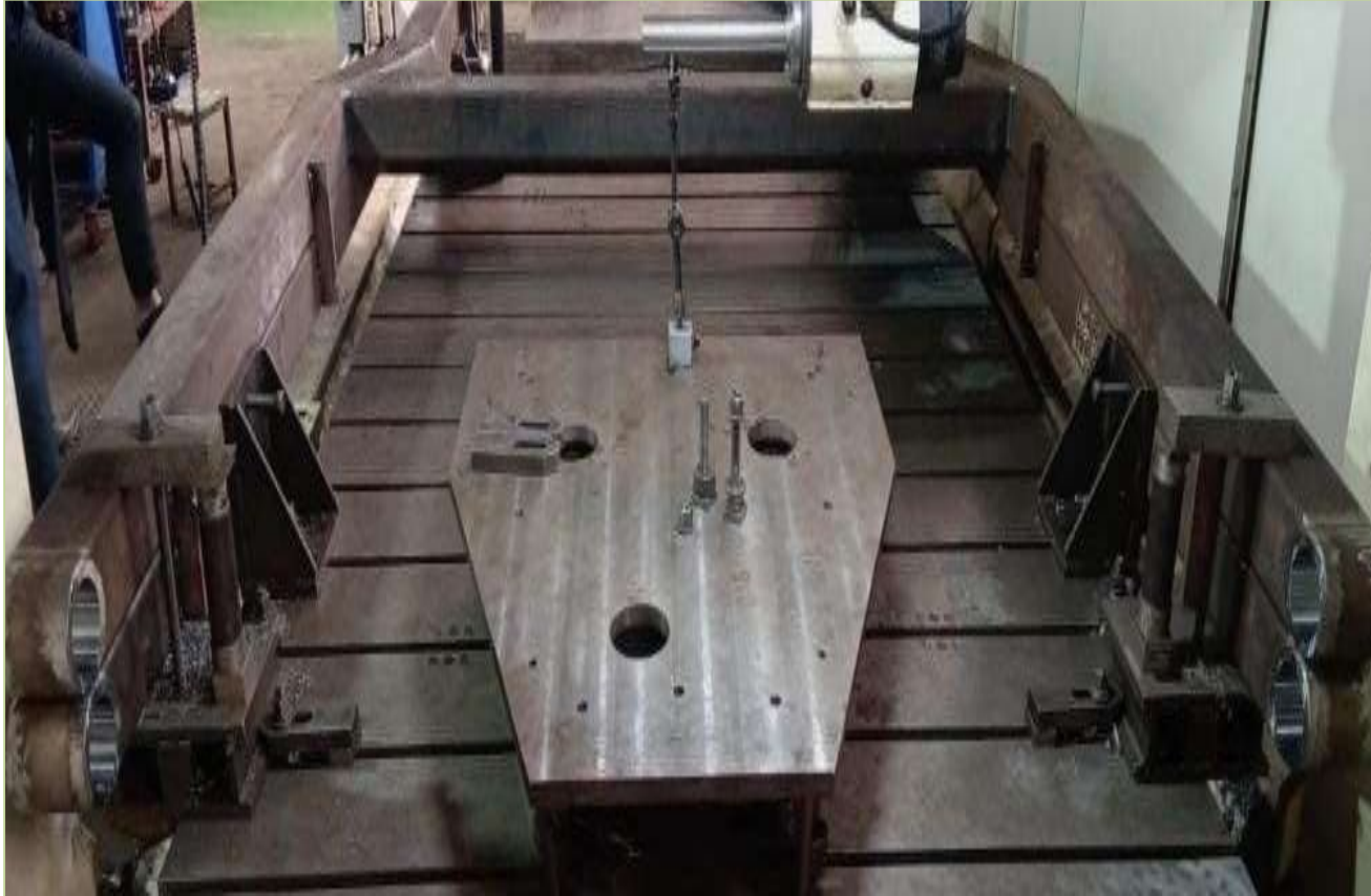
Rohini Radar System-Upper & Lower Linkage -Material-SA 516 GR 70
