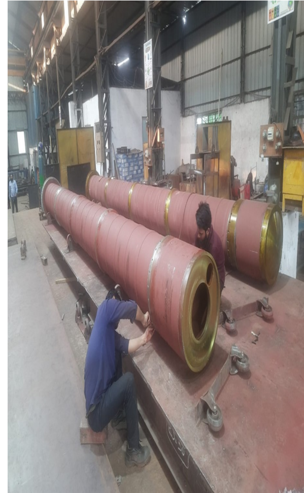
LRLACM : DUMMY CANISTER MATERIAL:- IS 2062 E250 GR BR / SIZE:- 8000 X Ø800
