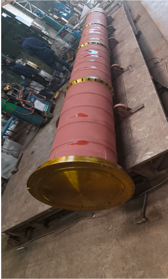
LRLACM : DUMMY CANISTER MATERIAL:- IS 2062 E250 GR BR / SIZE:- 8000 X Ø800
