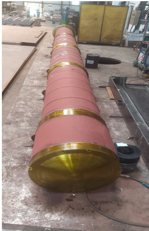
LRLACM : DUMMY CANISTER MATERIAL:- IS 2062 E250 GR BR / SIZE:- 8000 X Ø800
