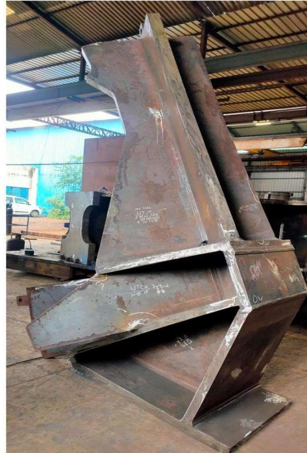
Corner Brackets -3050 X 1930 X 1550- Material EN10029-S355J2+N
