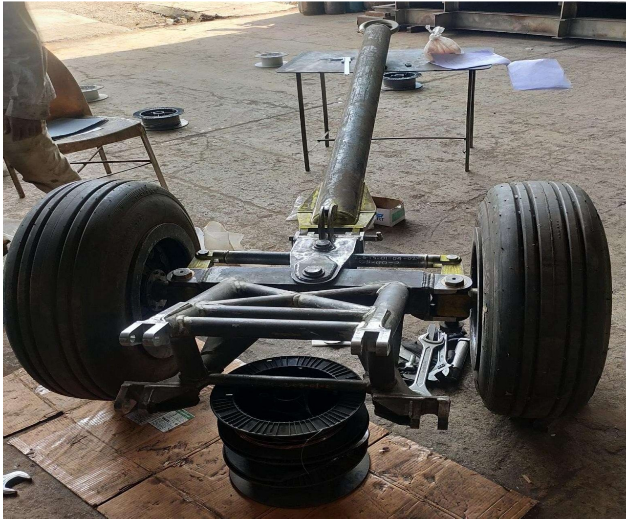
HDPS Front Wheel Carriage Assembly Material- S690QL , SA 106 Gr B
