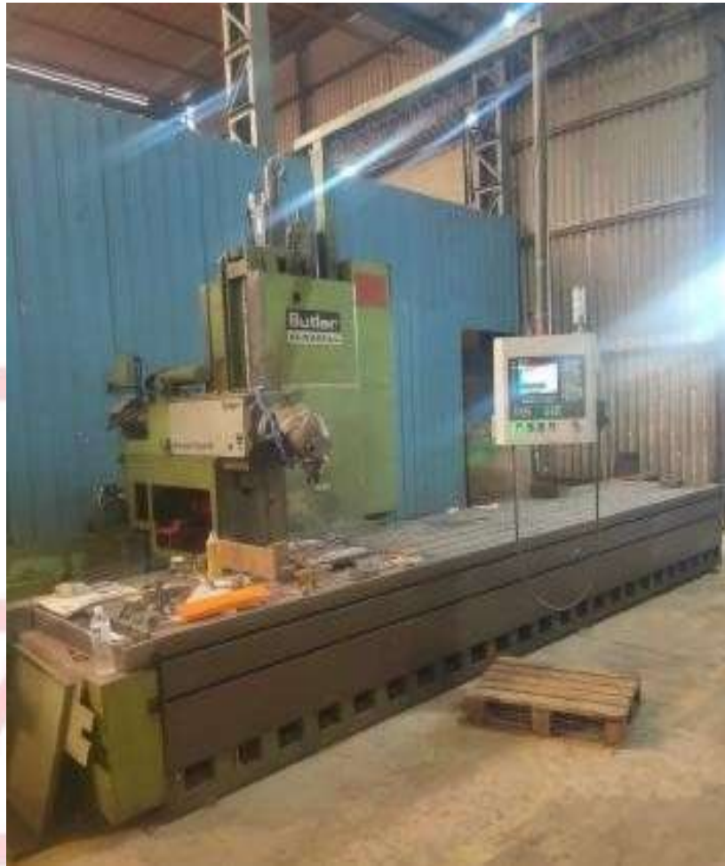
Horizontal Machining Center with Universal Head Make-Butler Hi-Power Elgamill
