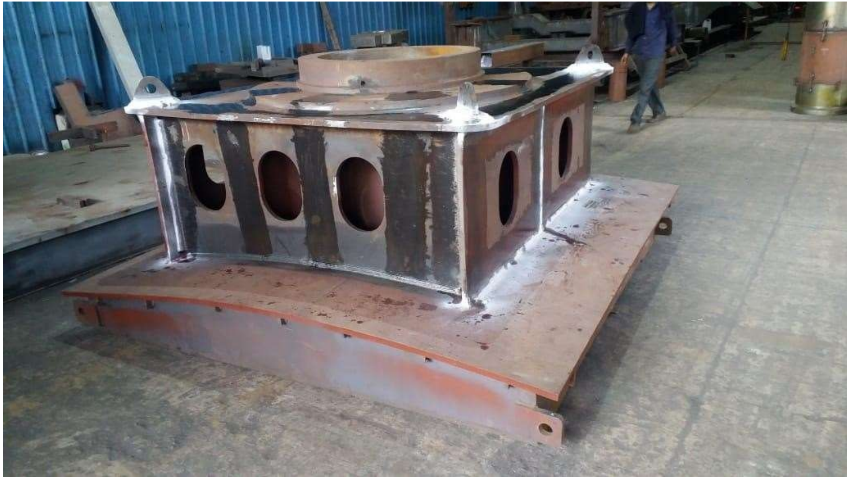
Steering Gear-STBD & PORT-Material DMR 249A
