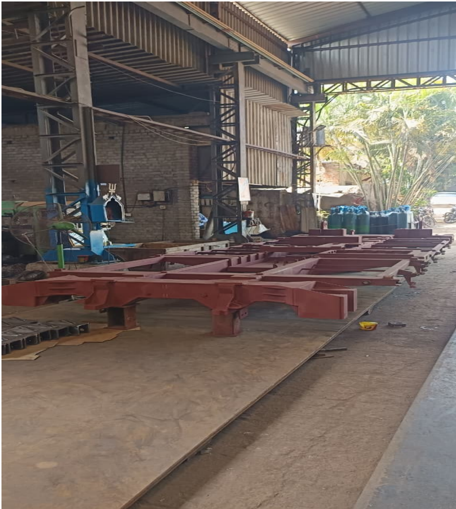
MRSAM & ASAM – UNDERFRAME STRUCTURE WELDED MATERIAL:- EN 10025-6-S690QL SIZE:- 8000 X 2286 X 1000
