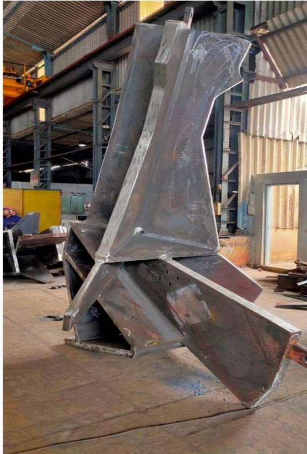
Corner Brackets -3050 X 1930 X 1550- Material EN10029-S355J2+N
