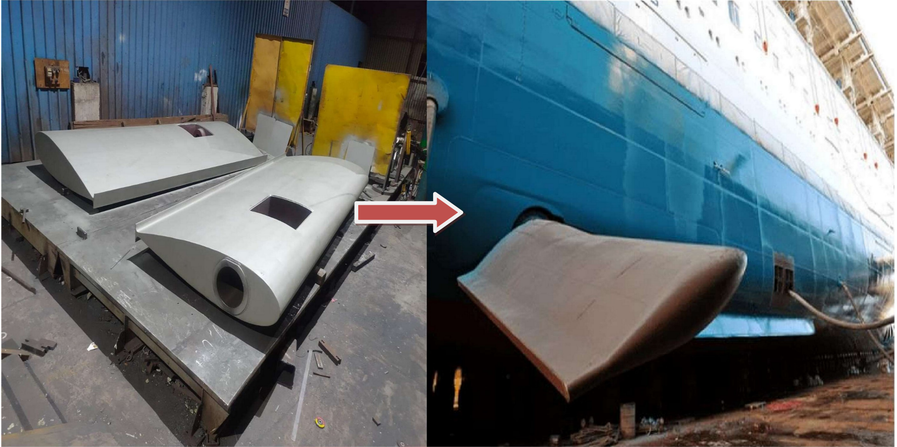
Ship Stabilizer- (FIN)-DSV-FIN-Material IS 2062 E350
