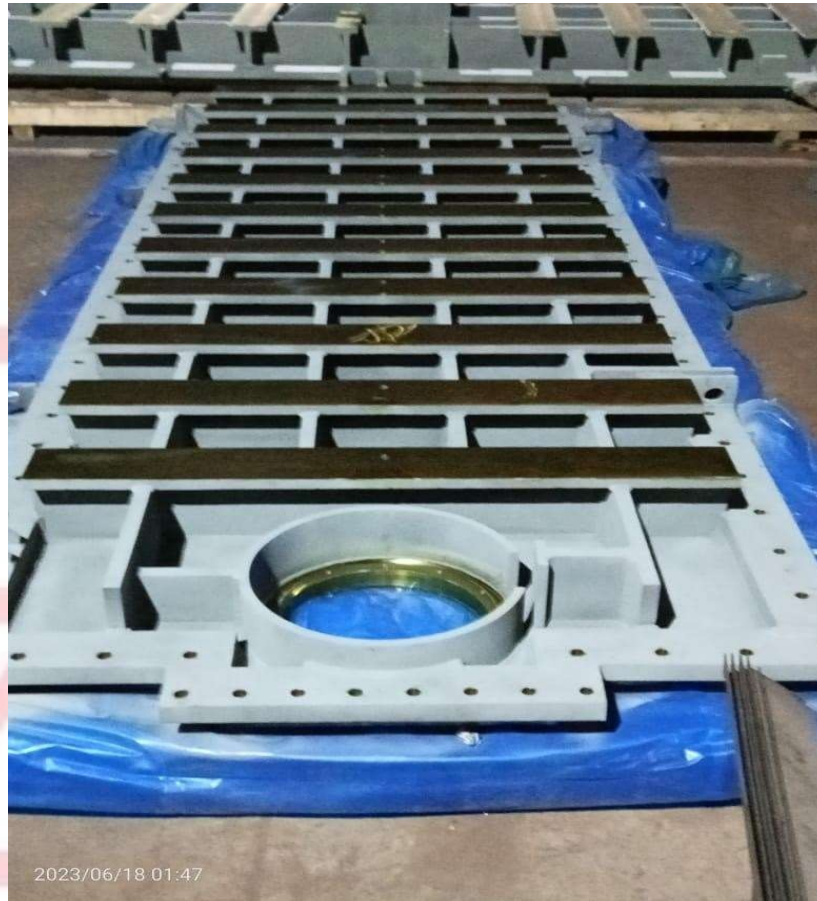
Side Wall for non-drive face- 5000 X 2000 x 350-Material : IS 2062 E350C
