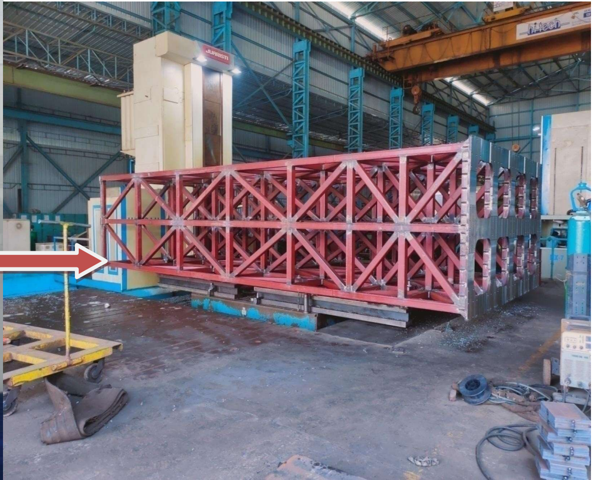
Universal Vertical Launcher Mechanism-Launcher Frame Assembly- 2100 X 4000 X 9000 mm;Material- DMR 249A (Refer next 3 pages)
