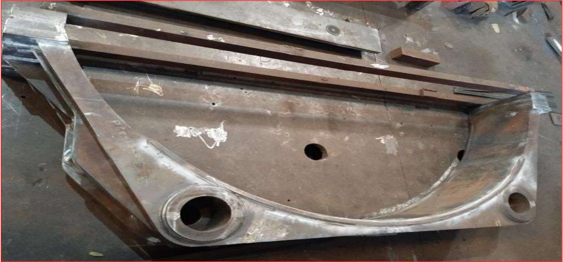
TCT- Cup Fabrication-Material- IS 2062 E450 & SA 508
