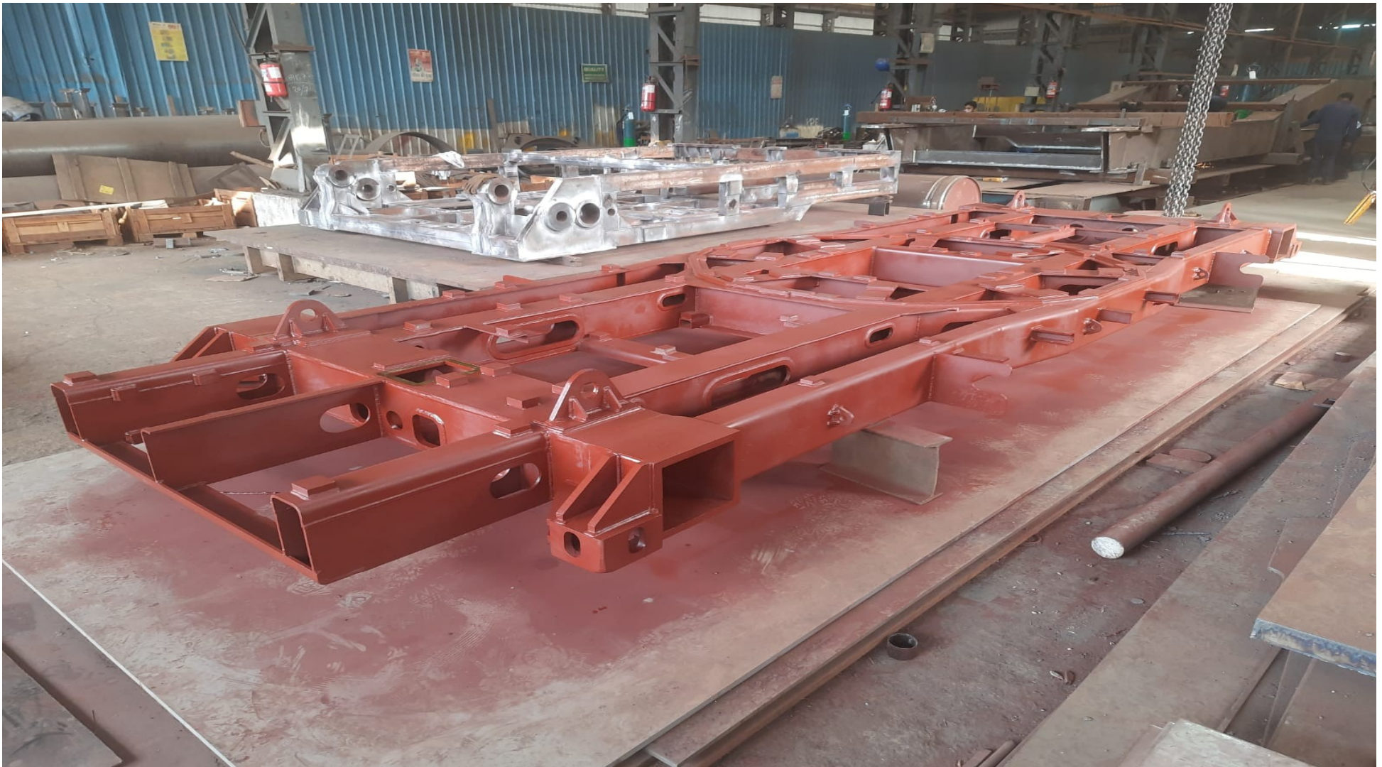
ARUDRA : PALLET STRUCTURE MATERIAL:- IS 2062 E250 GR BR / SIZE:- 6050 X 2600 X 300
