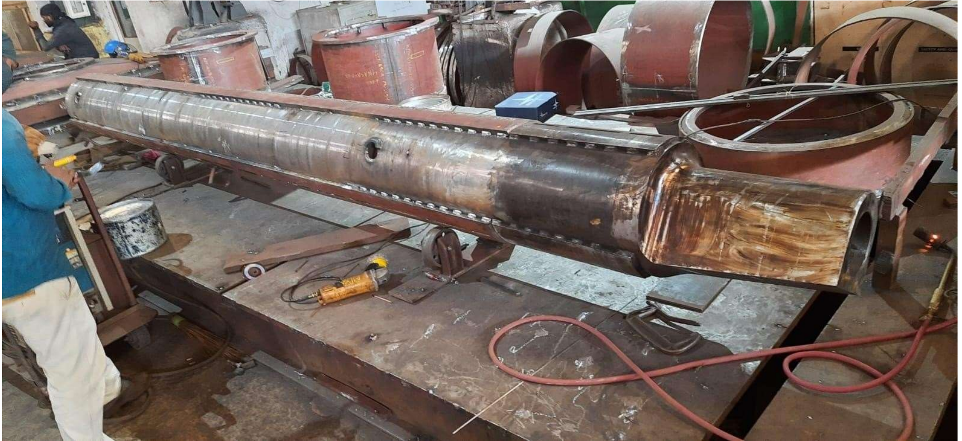
SG BEAM-Material DMR 249A , IS 2062 E250
